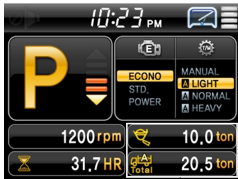
The example of the weighing system
