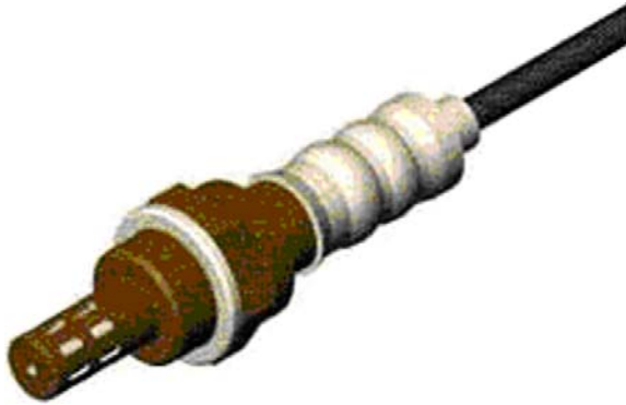
The Heat Exhaust Gas Oxygen (HEGO) Sensor
